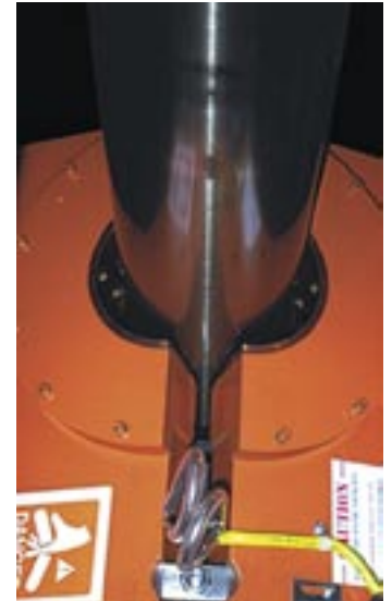
LifeJacket jaws in open position – normal operation.
